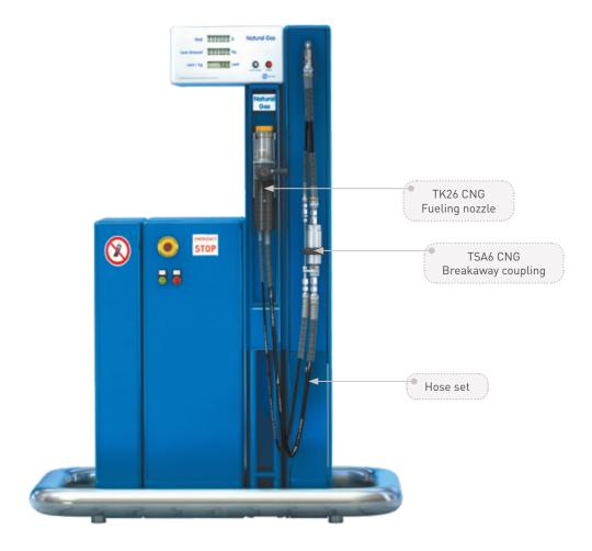
We also offer complete sets assembled and pressure tested for installation at fueling stations. The hose assemblies consist of a fueling nozzle, a hose set and a breakaway coupling. All hose assemblies are available with different hose lengths and can either be delivered with a type TSA1 CNG breakaway coupling directly mounted at the dispenser or a type TSA2 CNG inline breakaway coupling mounted inbetween the hoses.
