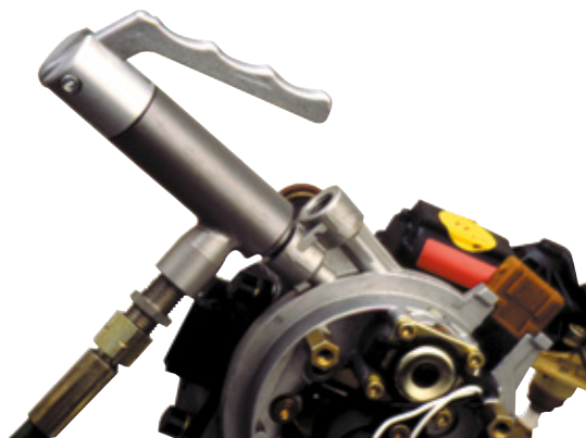
TW17H | Testing of injection pumps
