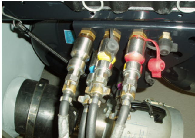
TW110 | For filling refrigerants in automotive air conditioning equipment during production
